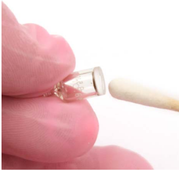
Figure 30: Polishing the Electrode Lamp Window
